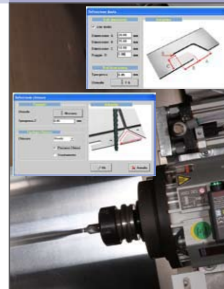
Milling tool, mounted on a ISO 30 cone, available in tool magazine, controlled by the routing unit
